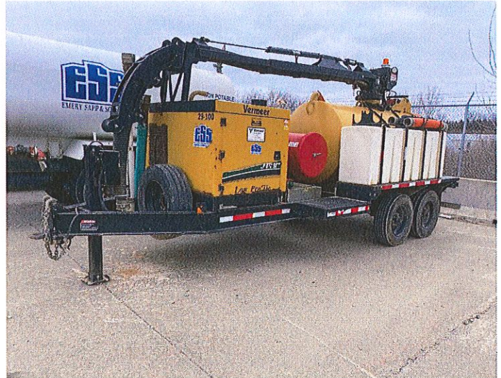
Vacuum excavation rig used by subcontractor, Emery Sapp & Sons
